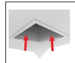
The diffuser can be installed by **gently** angling it and inserting up into the shaft.
