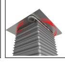
Using aluminium tape provided, secure flexi shaft to zincalume shroud at bottom of roof assembly.
